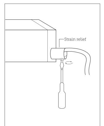
Connect the powerline to the power supply. The counterweight is 35 watt per meter. For example: for 2 meters of powerline a power supply of 70 watt is needed.
