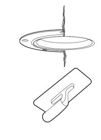
Note: Do not plaster higher than the inner edge of the plaster ring and prevent plaster from entering the ring.
